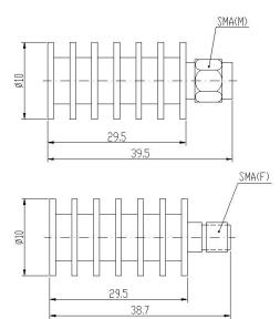
Coaxial fixed terminations absorb RF& microwave energy and are commonly used as dummy loads of antenna and transmitter. They are also used as match ports in many multiport microwave device such as circulator and directional coupler to make these ports which are not involved in the measurement be terminated in their characteristic impedance in order to ensure an accurate measurement.
